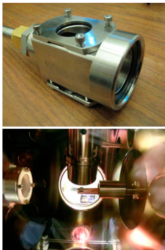
Figure 1. Pictures of the high-pressure cell (top) and overall arrangement (bottom) used in the operando studies. Top: high pressure cell, which consists of a small cylindrical cup fitted with an O-ring (right) to make a seal when pressed against the cylindrical piece of the manipulator and has two NaCl windows retrofitted to the side walls to let the infrared beam in and out of the cell during reaction (the holder for one of those windows is shown here on top). Also shown is the gas feeding and pumping tube placed at the back of the cell. Bottom: holding arrangement for the Pt crystal inside the UHV chamber, showing the stainless steel cylinder used to seal the high-pressure cell (right) and the two copper rods used to hold the sample. The cylindrical piece seen on the right of the bottom picture is used to guide the manipulator to the RAIRS position in the UHV chamber.
